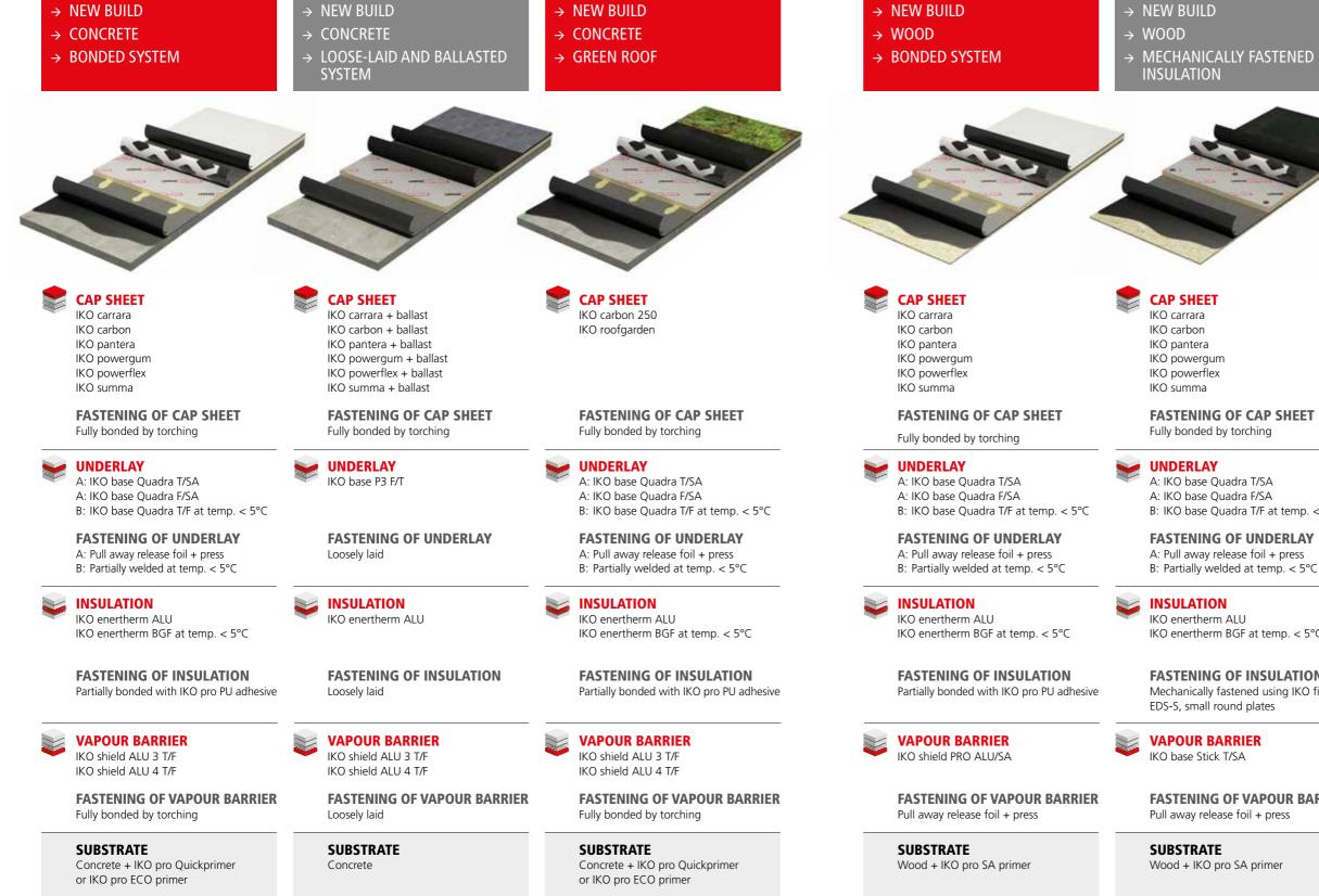
IKO pro Sprayfast or IKO pro PU glue can also be used for bonding the insulation boards.
