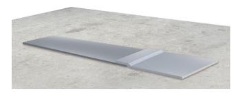
In both cases provide an overlap of at least 5 cm and absolutely avoid air entrapment.
