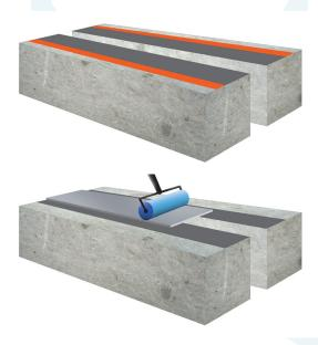
Stick the masking tape in the middle and over the entire length of the EUCO-JOINT B (width equal to the width of the joint or crack). Also reapply masking tape on the outer edges. Then spread EUCOCOL EP WS with a spatula or trowel over the first layer of EUCOCOL EP WS and over EUCOJOINT B. Then remove all masking tape.
